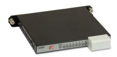
The F809F Fieldbus Diagnostic Module is available as an option for use with F800 Series and some F600 Series fieldbus power supplies. It plugs into the F8x0 or F6x8 Series power supply carrier or F8x8 diagnostic module carrier and monitors the performance of each of the eight fieldbus segments, providing information on the network health and capturing retransmissions between the fieldbus devices and control system.
