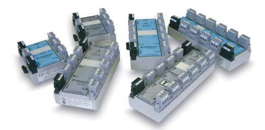
Megablocks are DIN-rail mounted passive hubs for FOUNDATION<sup>™</sup> fieldbus networks. They connect several field devices to the network trunk cable and provide short circuit protection to the segment. Megablocks minimize hand wiring and allow individual devices to be added to and removed from the segment without disrupting network communication.
