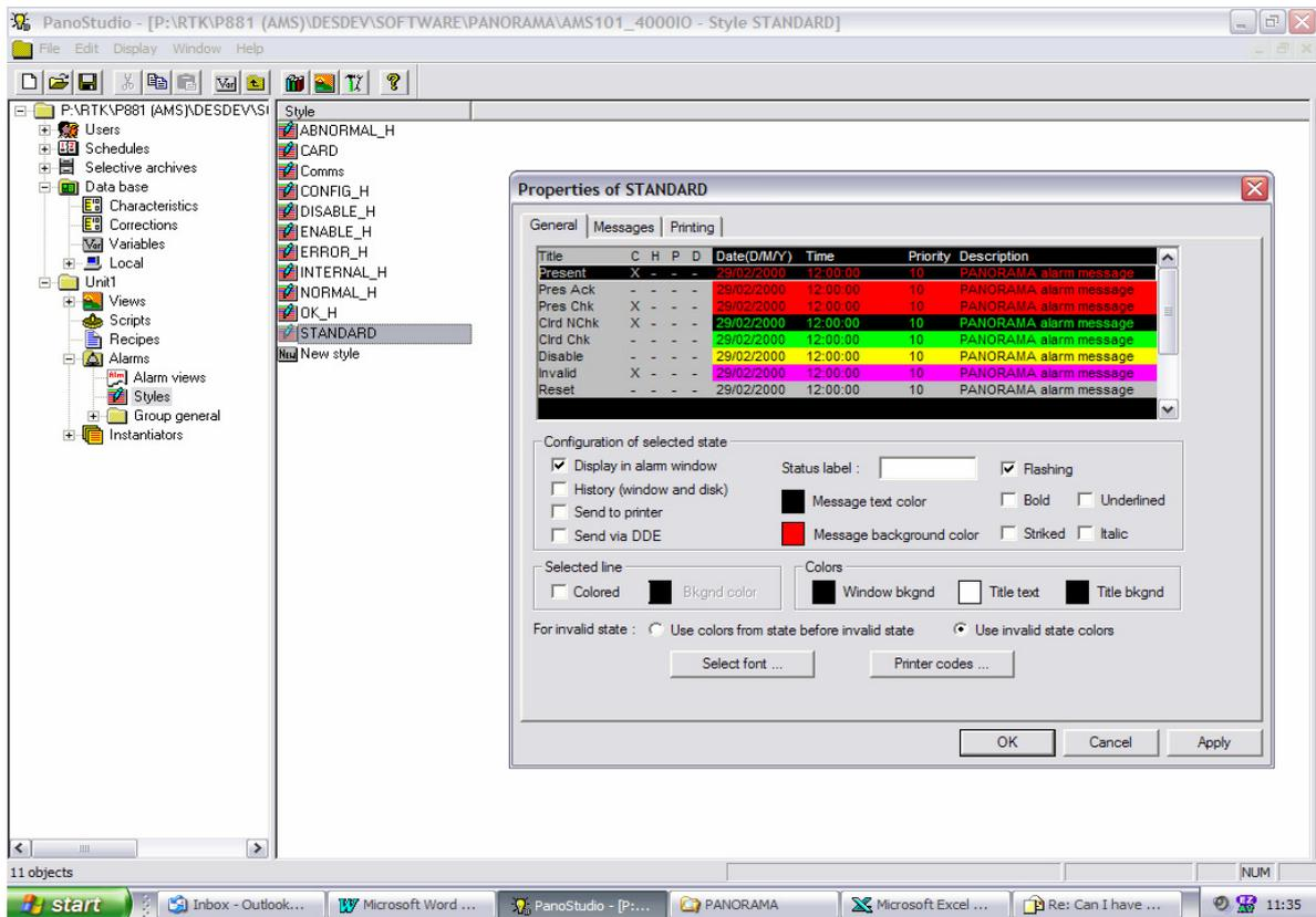
Under the General tab select the Title row labelled Cird Chk and in the Configuration of selected state area check the box labelled Display in alarm window as shown above.
