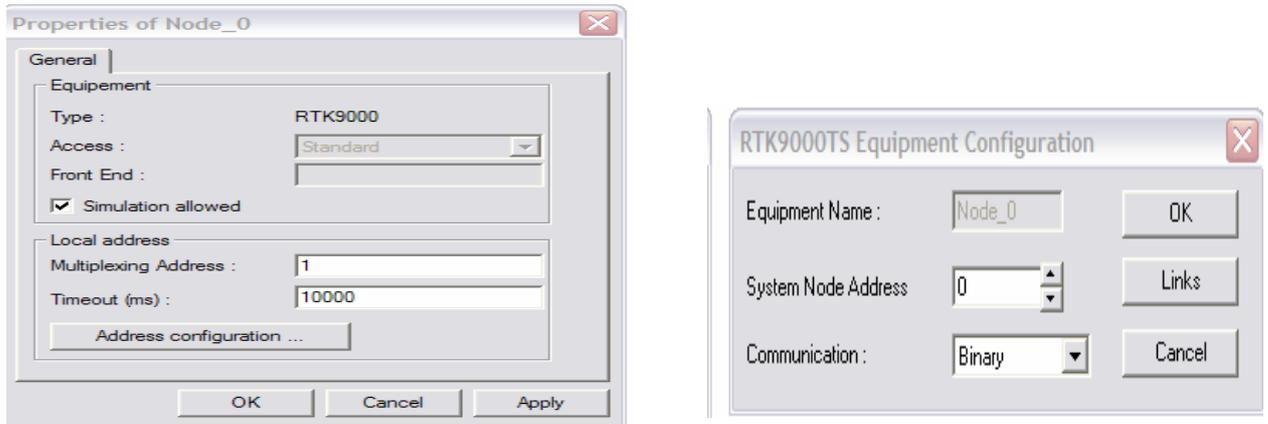
Select the Links icon within the RTK9000TS Equipment Configuration Menu to access the “Link Configuration- Node\_0” Menu as shown below.
