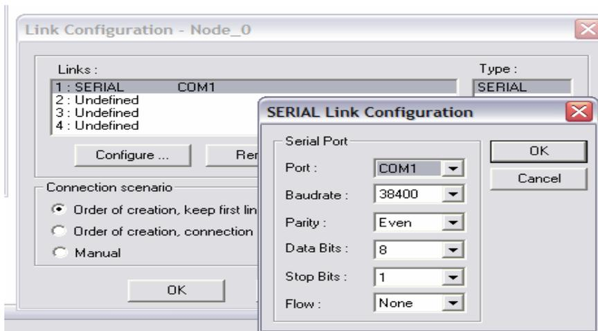
Select Link 1 SERIAL followed by the Configure icon to access the SERIAL Link Configuration Menu and note that COM 1 is always set as the factory default.
