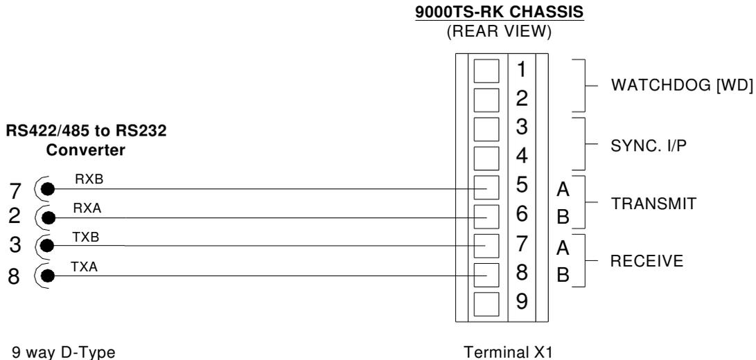
The System 9000TS can also be used with a RS485 device server which can be connected to the network via an ethernet connection. This can then allow any machine on the network to run the AMS software. The diagram below shows connections to the N-Port DE311 device server, set up as a RS422 connection.
