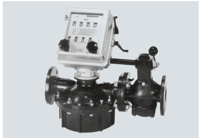
Automatic batch meter DN 50 (2"), with rotary-piston meter, quantity pre-set register and shut-off valve
