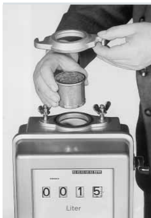
Quantity preset register with desiccant cartridge removed
