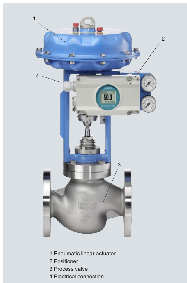
Positioner, attached to linear actuator
